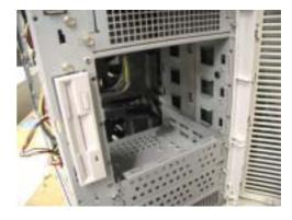
**f.** Remove four screws, and remove the SCSI-B.P. (with SAF-TE board) gently away from the disk cage.
